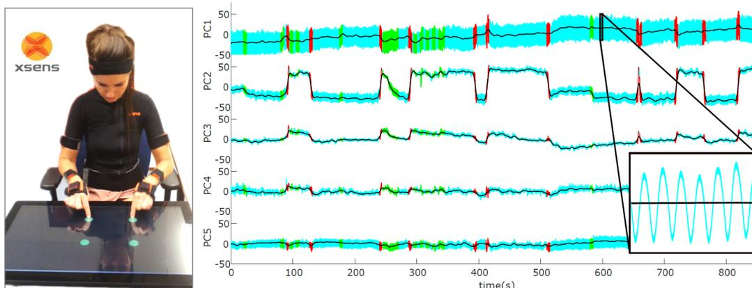
**Fig.1** Left: experimental set-up. Right: Dataset of a 15-min trial of one volunteer: the first 5 PCs are shown. The tapping movement is printed as a colored line, the black line represent the low-pass filter underlying trend. Quasi-stationary phases were colored in cyan,
